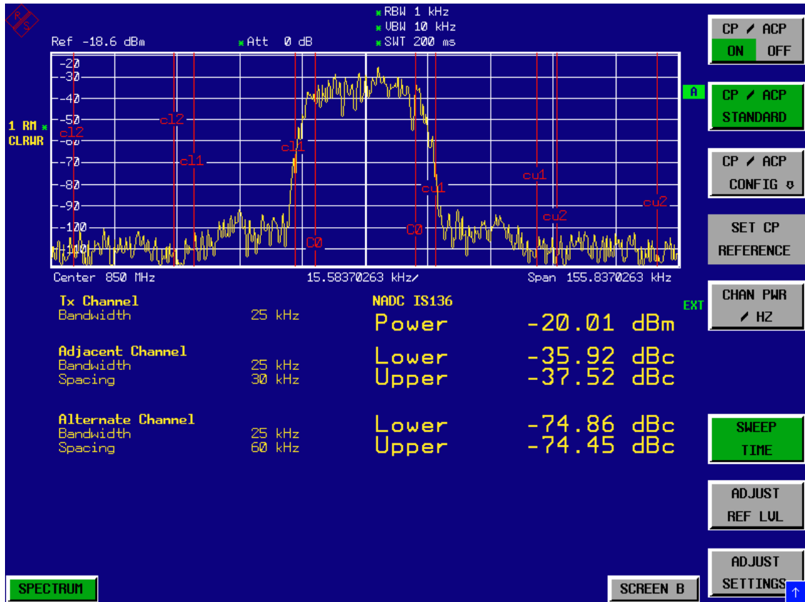
Fig. 2.27 Measuring the relative adjacent channel power of an NADC signal in each of the two adjacent channels below and above the transmit channel.
